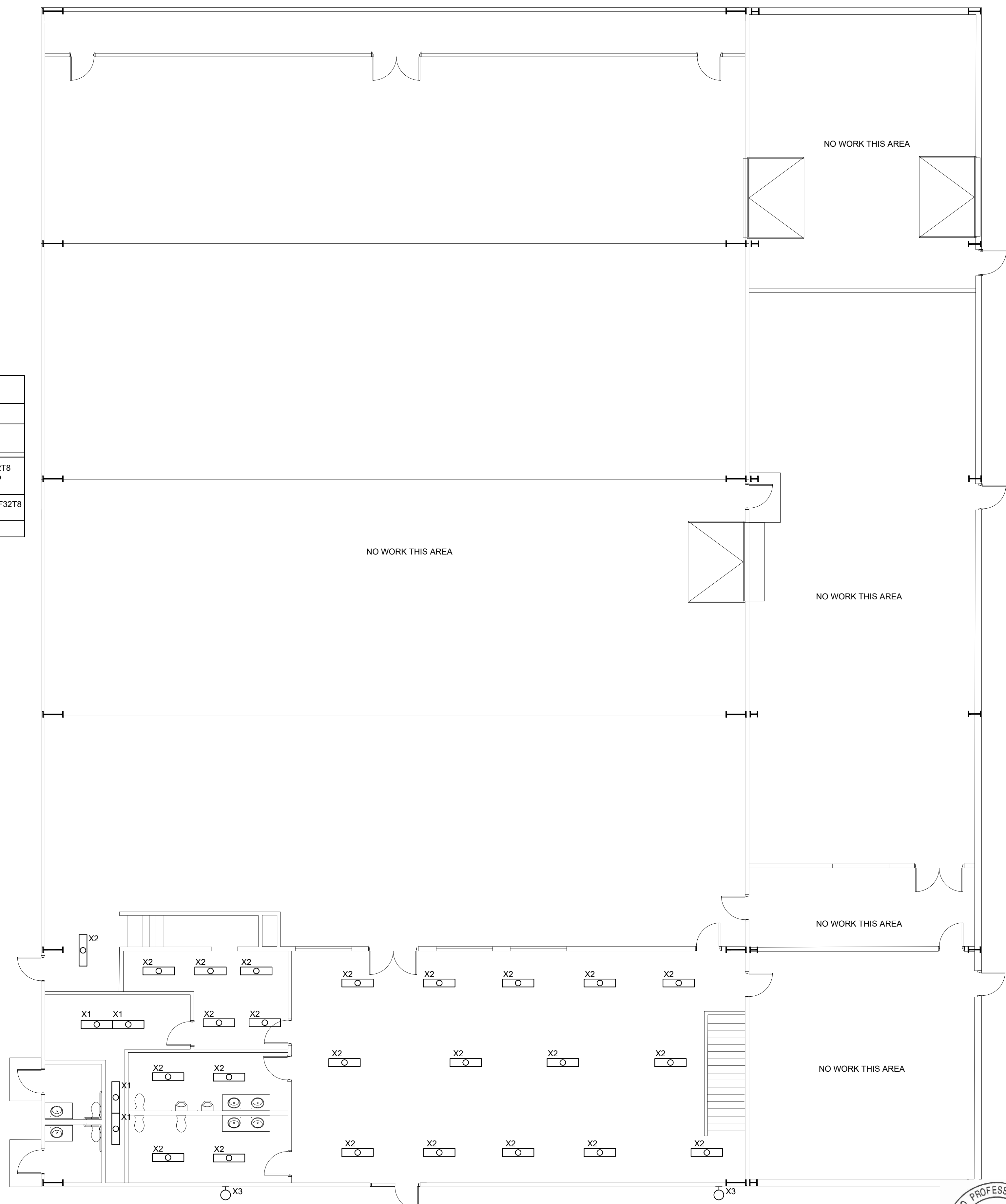
1 Main Level Lighting Demolition Plan 1/8" = 1' - 0"
